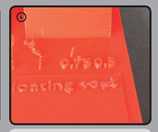
Some details are not connected to the main 3D model.
