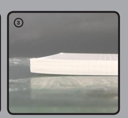
The base of the model is warped.
